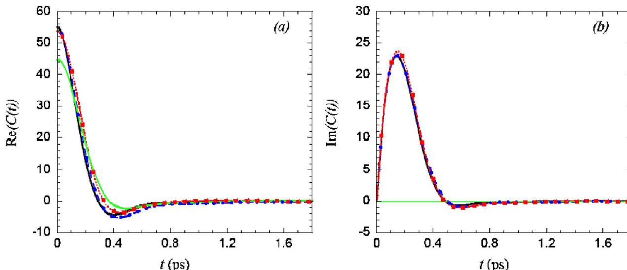
FIG. 4. (Color online) The velocity autocorrelation function of liquid neon. panel (a) shows the real part of the correlation function while Panel (b) depicts the imaginary part. Black solid line: PP-FBSD result. Blue solid circle with dashed line: TGA-LSC-IVR result. Red solid square with dotted line: TGA-FBSD result. Green solid line: classical result.
