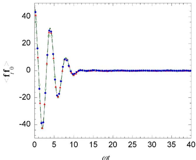
FIG. 2. (Color online) The symmetrized force autocorrelation function for the one-dimensional anharmonic oscillator given in Eq. (5.1) for  $\beta\hbar\omega = \sqrt{2}/10$ . Black line: Exact quantum mechanical result. Green hollow square with dashed line: classical result. Red solid triangle: TGA-LSC-IVR result. Blue solid circle: TGA-FBSD result.
