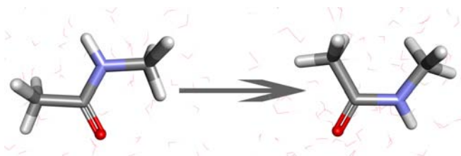
FIG. 1 Model system (ACE-NME) in water. The backbone C–C–N–C dihedral is used as the reaction coordinate for describing the dihedral flipping.
